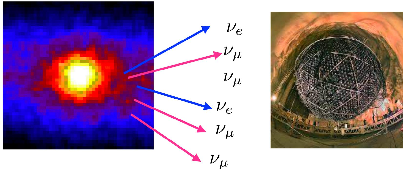
SNO 1 ton heavy water ( $D_2O$ ) tank surrounded by 9600 PMTs. Deuterium has binding energy 2.2 MeV  $\implies$  SNO can detect Boron 8 solar neutrinos.
