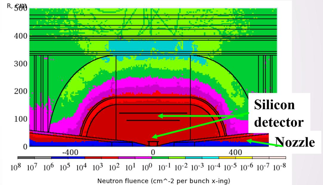
Neutron maximum fluence and absorbed dose in the innermost layer of the Si tracker for a one-year operation are at a 10% level of that in the LHC detectors at the nominal luminosity.
